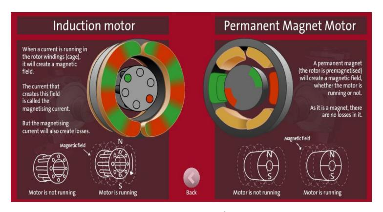
\* An ECM motor uses approximately 50% less energy than a comparable standard induction motor
